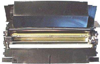
Toner cartridge with corona wires exposed
